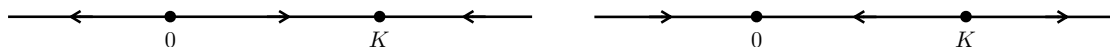
Figure 2.3: Phase portraits of the logistic equation (2.21) for r, K > 0 (left) and for r < 0 < K (right). The flows defined on the same phase space X = [0, K] are not topologically equivalent.
